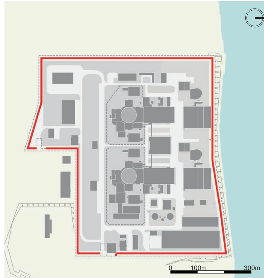
1 Hinkley Point C site arrangement currently under construction due for completion in 2025. Footprint of operational site inside secure fence line and excluding National Grid substation is approximately 46 ha.
